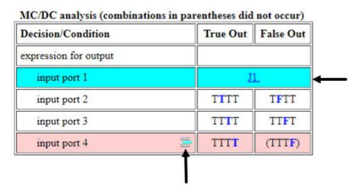
The input port 1 expression is a missing coverage objective that has been justified after MCDC analysis. The input port 4 expression shows a missing coverage objective and the **Add justification rule** icon.
