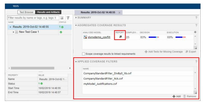
From coverage results. You can create new filter rules from a coverage report by right-clicking a block with model coverage highlighting or from the **Coverage Details** pane. For more information, see View Coverage Results in a Model.
